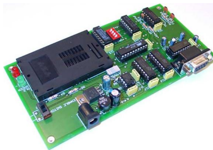
Figure 3: An “unlooper” device makes use of fault injection (US$ 100)
